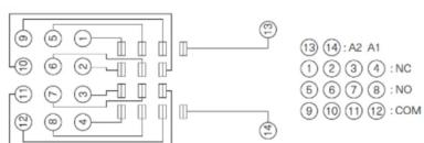
SOCKET GS 4C-PU Wiring Diagram
