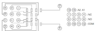
SOCKET GS 4C-PU Wiring Diagram
